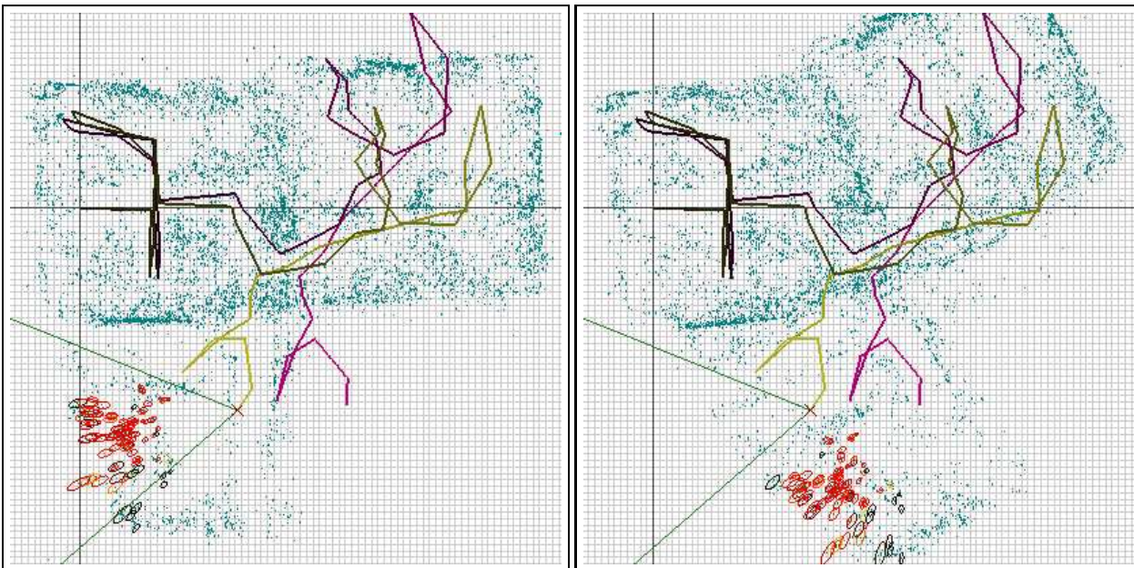
Figure 4. Left: The constructed map for the best sample at the end of exploration. Yellow: maximum weight trajectory. Pink: Dead reckoning trajectory. Grid lines indicate 25cm intervals. Right: the constructed map using dead reckoning.
