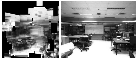
Figure 1. Left: A rendering of the map from a sensor's-eye view. Right: an image of the lab from a nearby position.
